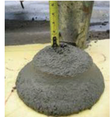
Slump Test
